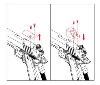
When installing the reddot screws to be attached to the reddot, we recommend using threadlocking fluid.
