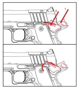
The hammer safety is engaged when the hammer is cocked and the thumb selector lever is switched into the up position. When the hammer is not cocked, this safety cannot be engaged, however, it can be engaged if the hammer is half-cocked.
